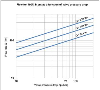
The flow tolerance for standard servovalves is  $\pm 10\%$  of the rated flow at 100% rated input signal.
